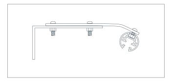
**Top brackets.** This adjustable fixing bracket is fixed to the top of the trough light and protrudes from 116mm to 204mm max.
