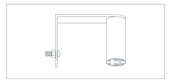
**Side brackets.** These attach to the side of the trough light and protrudes 50mm - 100mm from the wall (depending on customer specification)
