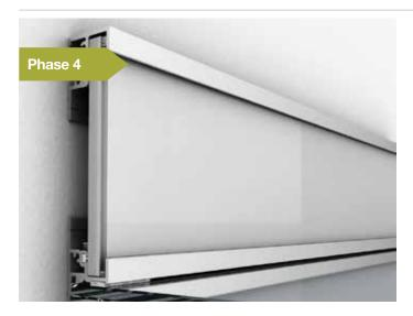
4. After positioning the supporting structure, the shelves are inserted. The inclination of the shelf can be adjusted by tightening the grub screws (see step 2) with an Allen key.
