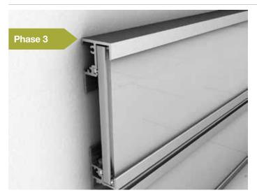
3. Next install the top profile. First fit the wall support Z-Vario (or length of z-section) onto the wall and then place the top profile on top, slotting it over the LED Light Sheet panel.
