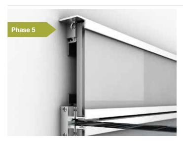
5. Using self tapping screws, side brackets with Velcro are secured to ends of intermediate profiles and top/bottom brackets are secured to the top/bottom profiles.
